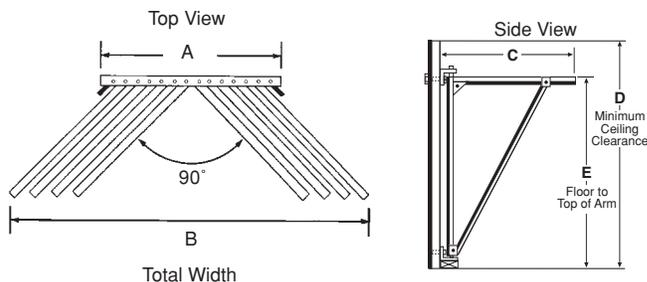
**IMPORTANT:** Have your architect, contractor or structural engineer certify your structural load-bearing wall. Our Multipost system offers a perfect alternative when load-bearing walls are not available. See information (page 9F) to incorporate our Multipost system for a wall-style installation or refer to Floor Models (page 3F). Be sure to involve your architect or structural engineer.
